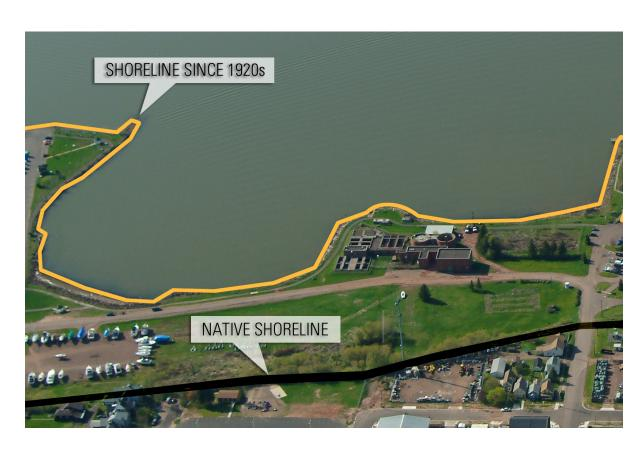
By constructing all or part of the outer perimeter of the Permanent Engineered Shoreline as a bulkhead wall, a new vertical shoreline would be established that could be designed to accommodate access and docking by vessels and public boats. Similarly, a boat ramp could be incorporated to augment the Prentice Avenue boat ramp at a similarly accessible point.
